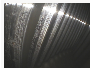
Working Flank - 8 year old thru hardened ring gear
