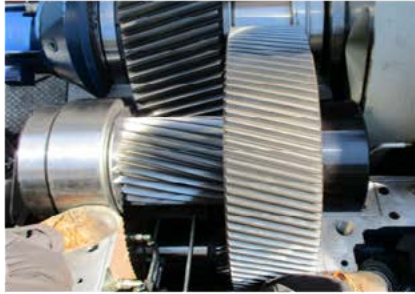
Picture 7. New IMS installed.
