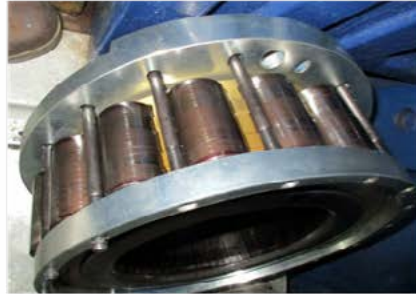
Picture 5. Damaged HSS RS bearing.
