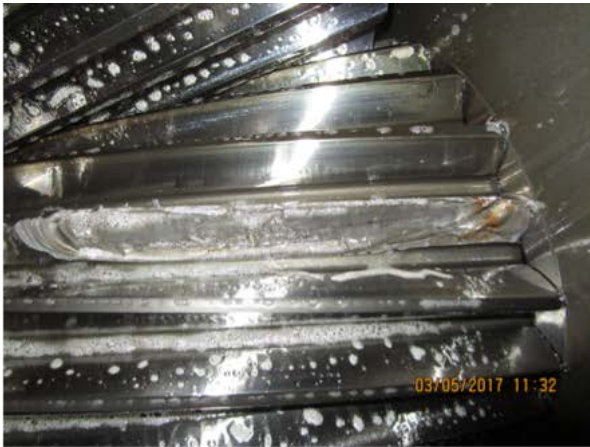
Picture 1 Broken tooth of IMS pinion.
