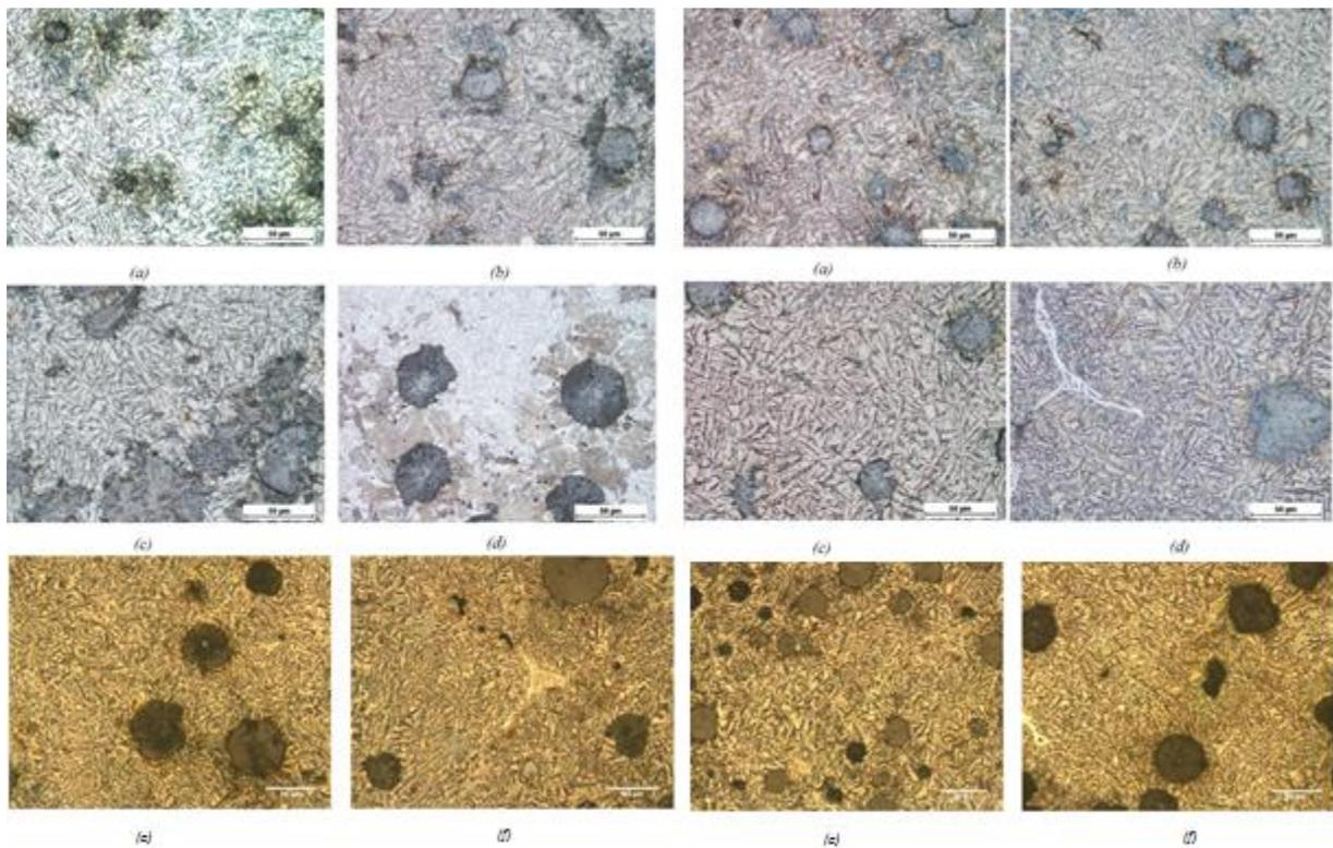
**Figure 7:** ADI samples (ADI-2 left, ADI-3 right) etched with Nital (2%) and numbered from 1-6 at (a) 10 mm and 75 s etching time, (b) 45 mm and 75 s, (c) 90 mm and 75 s and (d) 150 mm and 75 s and samples 5 and 6 etched with Nital (5%) at (e) 255 mm and 6 s etching time, (f) 290 mm and 6 s and depth starting from the chilled side. Pictures were taken with a 50x objective.
