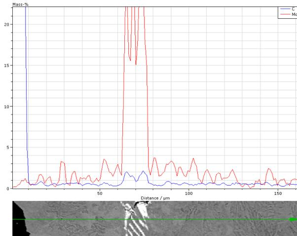
**Figure 8:** EDS line scan analysis measured starting from a graphite nodule through a Mo-carbide.
