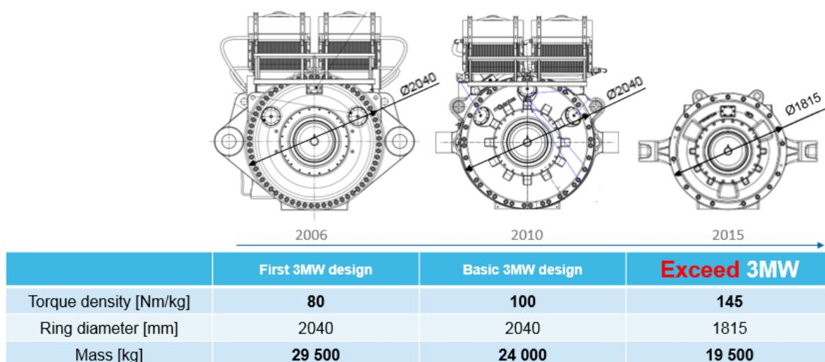
**Figure 1:** The evolution of 3MV gearbox from 2006 to 2015 showing the decrease in mass along with increased torque density
