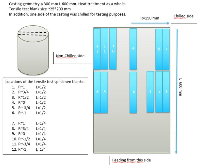
**Figure 2:** Initial design geometry and test sample locations
