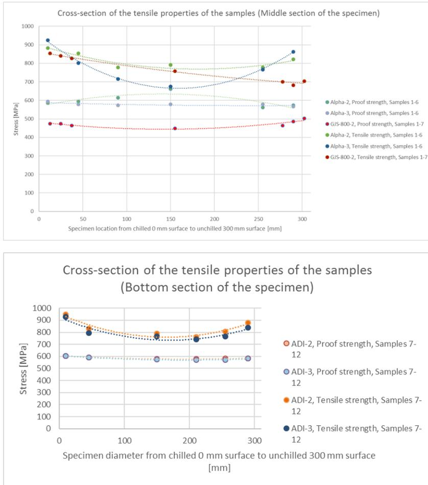
**Figure 3:** Tensile properties for the middle and bottom cross-section of the specimen, measured from the chilled to the unchilled surface.
