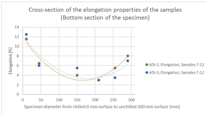
**Figure 4:** Elongation properties for the middle and bottom cross-section of the specimen, measured from the chilled to the non-chilled surface.
