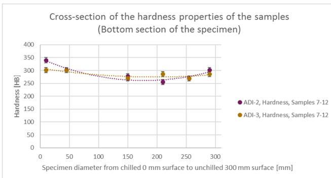
**Figure 5:** Hardness properties for the middle and bottom cross-section of the specimens, measured from the chilled to the non-chilled surface.
