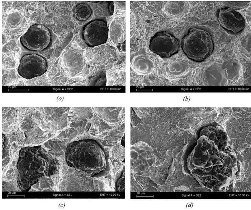
**Figure 6:** Fracture surfaces of ADI-2 samples at (a) 10 mm, (b) 45 mm, (c) 90 mm and (d) 150 mm depth starting from the chilled side.
